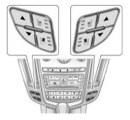
If available, the buttons are near the climate controls on the instrument panel. To operate, the ignition must be in ON/RUN/START.
